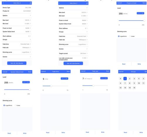
Step 5: After setting, please save the selected configuration via NFC and power on the device.
